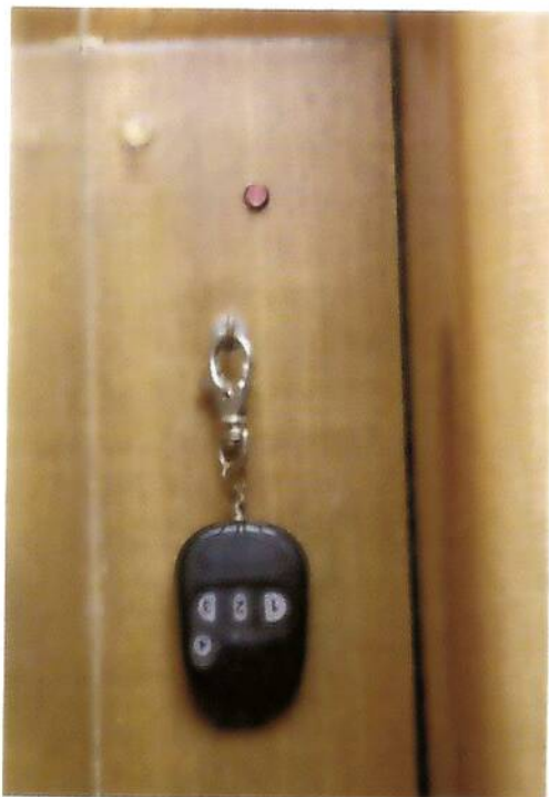
Alarm remote control for enabling and disabling the system and flashing LED by the companionway. We keep a remote by the companionway and one by our bed.
